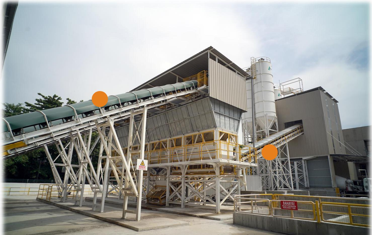
● Conveyor top covers to minimize dust emission into the atmosphere
