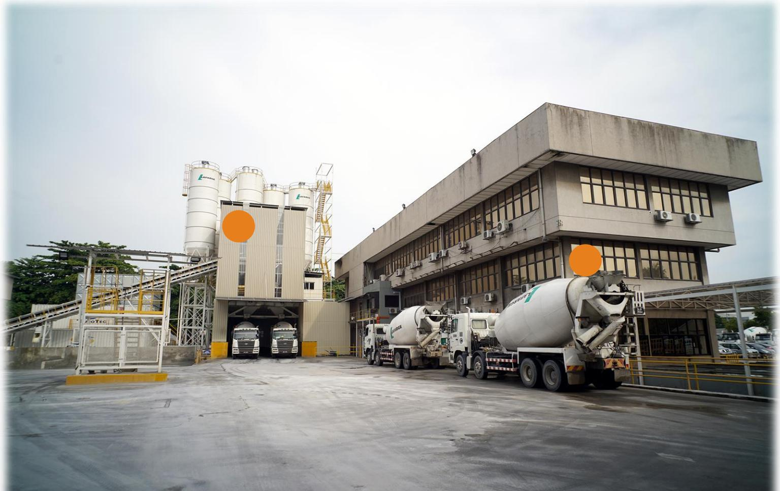
Enclosed batching area to minimize dust emission into the atmosphere
