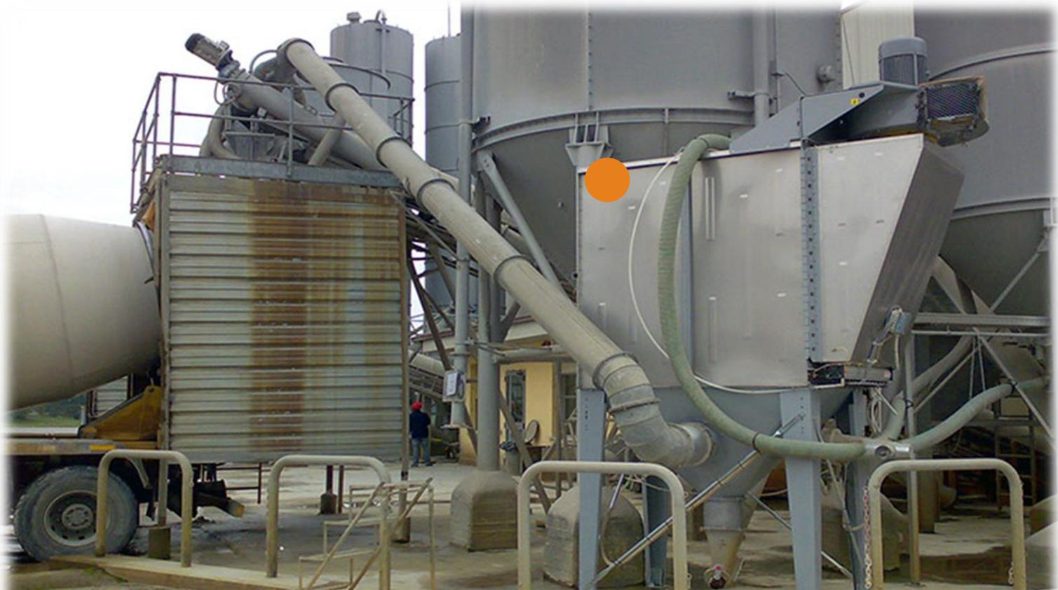
Dust collector is designed for dust collection from the truck mixer inlet zone in dry batch plants during loading of the truck mixer drum/agitator
