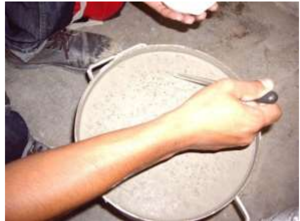
Bleeding Test on fresh concrete mix (BS EN 480-4)
