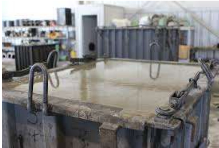
Figure 1. Excessive Bleeding in Freshly Cast Concrete.
