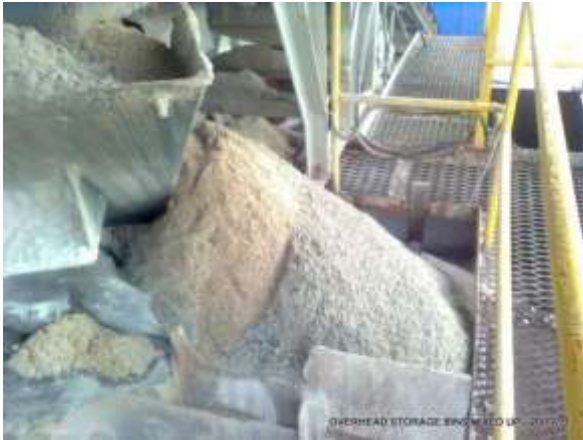
Cross contamination in material storage hopper
